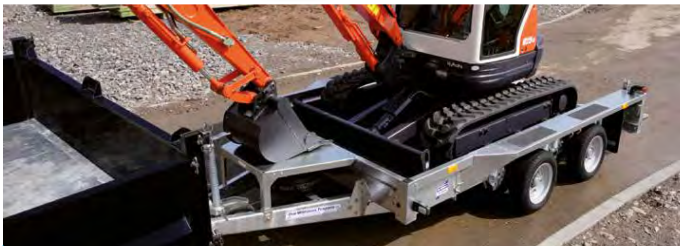
GX106 with skids and integrated rear supports
